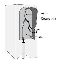
**Step 2**: Wire the keypad to the gate opener control board. Strip 3/16" off the ends of one pair of low voltage wires. Attach the wires to the terminal block marked RELAY on the keypad control board as shown. Then connect wire #1 to the CYCLE terminal on the gate opener control board, and wire #2 to the COM terminal on the gate opener control board
